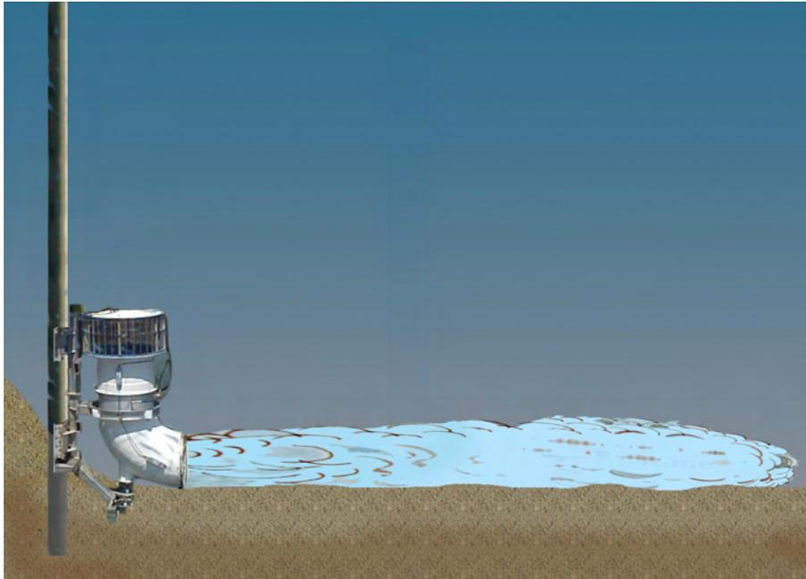
Figure 1: Water jet suspends sediment
