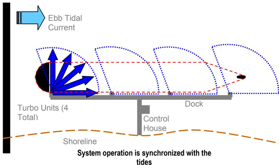
Figure 3: Operational diagram
